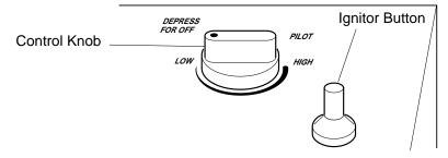
Figure 16 - Control Knob and Ignitor Button
